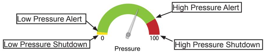
The System Pressure, Flow Rate, Post-Filter Pressure and pH Balance sensors provide warning zones on their UI dial indicators when displayed on the dashboard.
